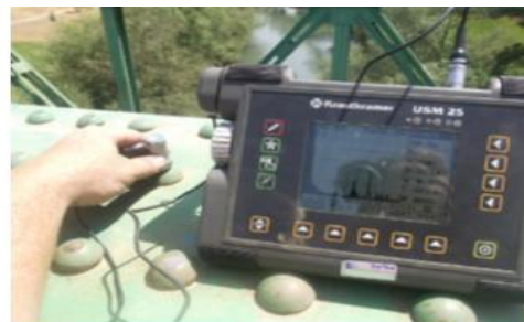
Fig. 40 Ultrasonic testing of rivets
