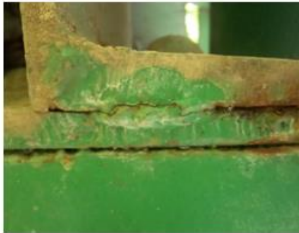
Fig. 25 Construction welding broken due to fatigue
