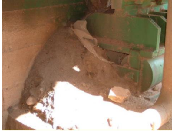
Fig. 33 Nonfunctioning roller bearing
