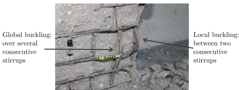
Fig. 3: Failure of an I-shaped column due to the global and local buckling of longitudinal bars
