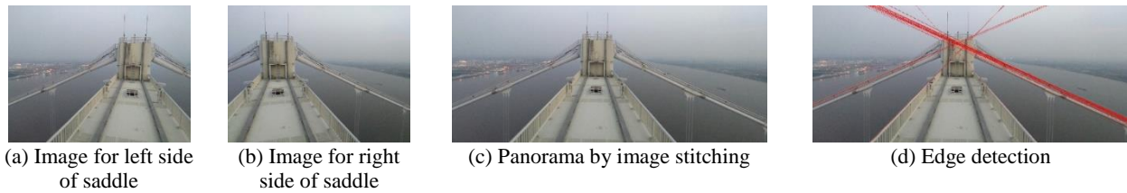
Fig. 9. Calibration of wrapping angle based on computer vision.
