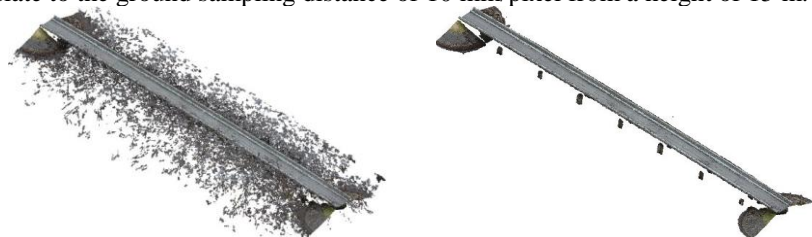
a) A point cloud generated from images b) A point cloud after removing noise data Fig. 3. A point cloud of the bridge from a image acquired from UAV
